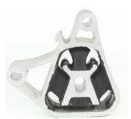
Figure 2 - The top engine mount
